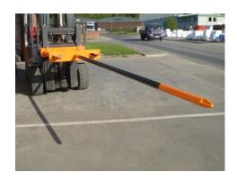
As with the Carriage Mounted Pole the **Fork Mounted Pole** is capable of lifting a variety of coiled products, but is usually used in low volume / occasion usage environment with a mixed pallet / coiled product application.
